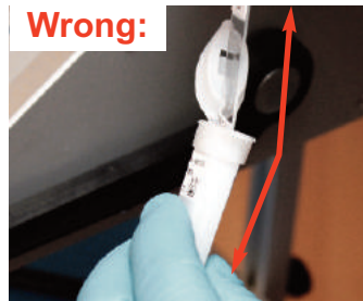
Figure 49 Position of the slide when taking or inserting it
