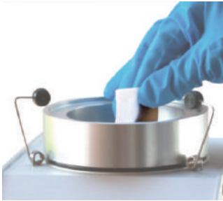
Figure 39 Cleaning the middle part
