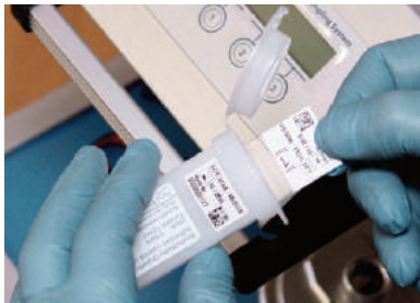
Figure 48 Taking the adhesively coated slide out of the container
