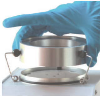
Figure 40 Taking off the sampling head
