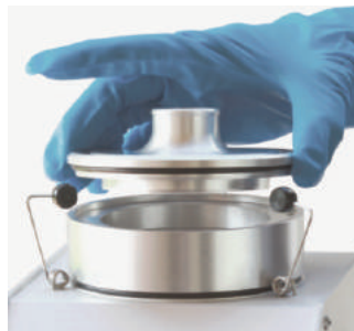
Figure 38 Taking off the top part
