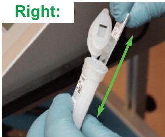
Figure 49 Position of the slide when taking or inserting it
