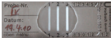
Figure 44 Completely overloaded particle tracks (cannot be evaluated)
