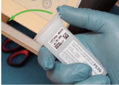
Figure 47 Opening the shipping container
