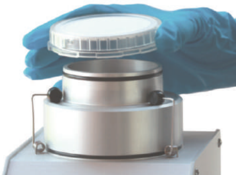
Figure 45 Mounting a gelatine filter in a single-use unit
